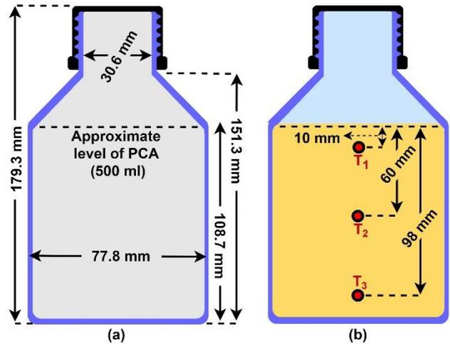
Figure 1. Shape and size of modeled bottle during computation (a), sensor locations on which temperature changes were monitored.
