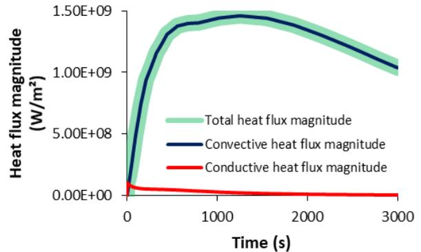
Figure 7. Heat flux magnitude calculated as convective, as conductive and as total vs time.
