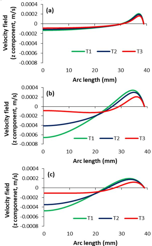
Figure 5. Velocity profile vs time and sensor location for time of 100 s (a), 1500 s (b), 3000 s (c).
