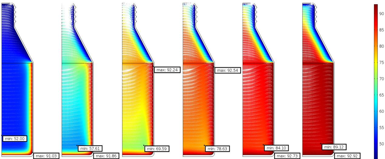
Figure 3. Temperature profile (°C) and minimum and maximum points in PCA medium in a glass bottle as a function of time for 100, 500, 1000, 1500, 2000 and 3000 s (left to right)
