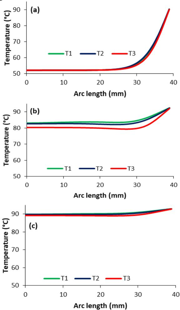
Figure 6. Temperature profile vs time and sensor location for time of 100 s (a), 1500 s (b), 3000 s (c).
