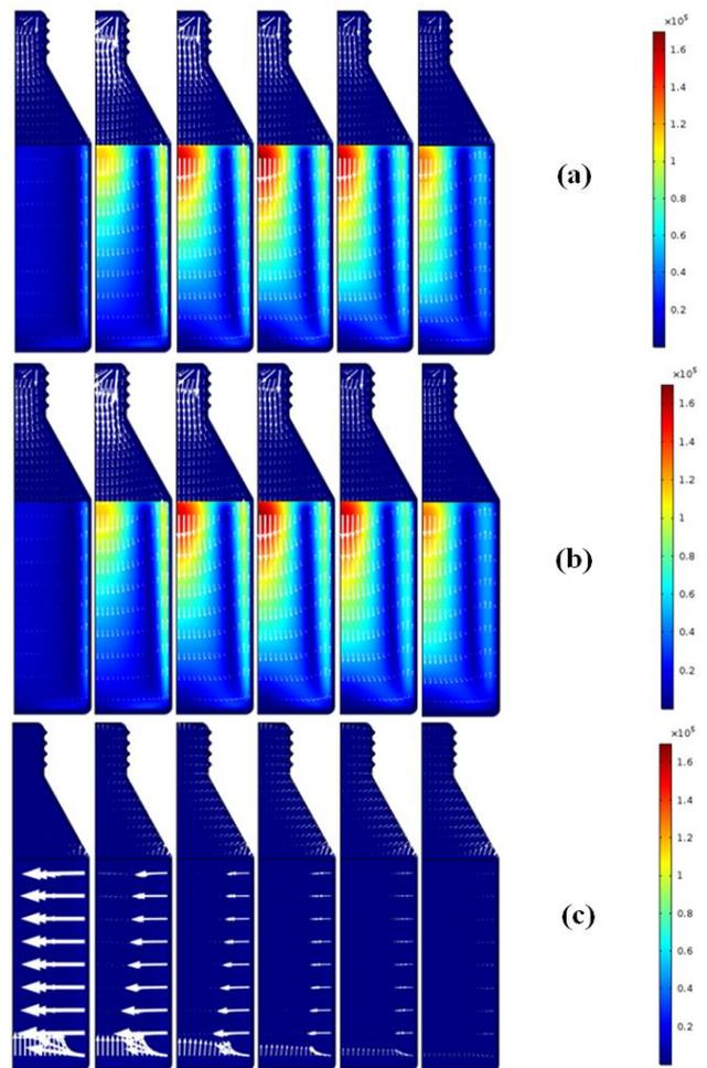
Figure 8. Heat flux magnitude ( $W/m^2$ ) over axisymmetric surface calculated as total (a), as convective (b) and as conductive (c) for 100, 500 1000, 1500, 2000 and 3000 s (left to right).
