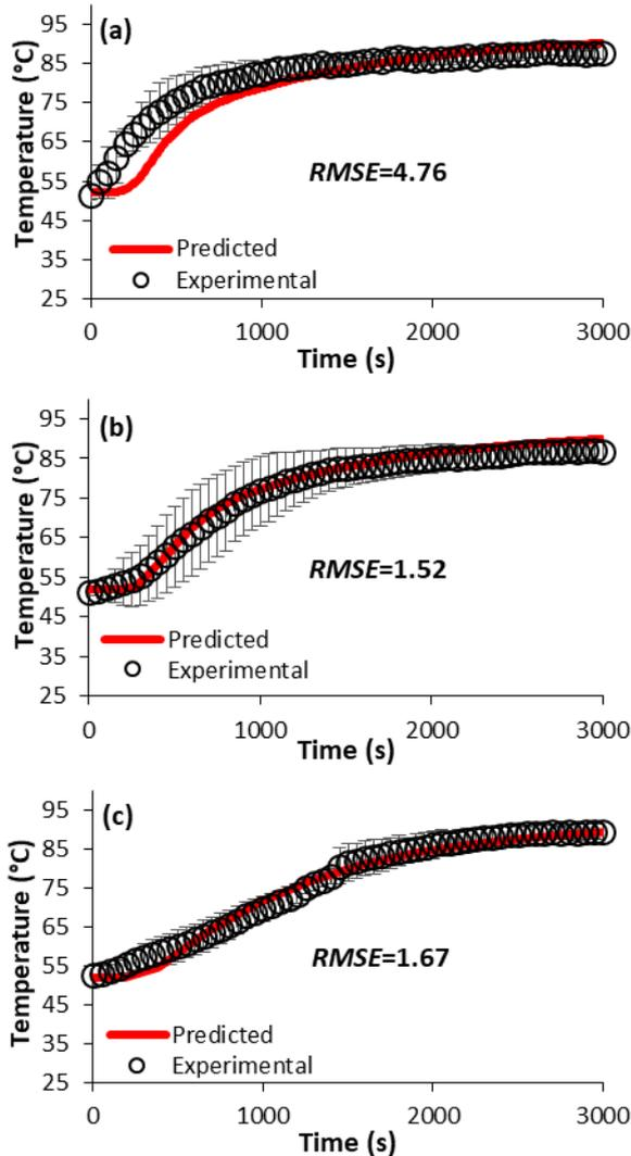
Figure 4. Temperature vs time at top sensor location (T<sub>1</sub>) (a), middle sensor location (T<sub>2</sub>) (b), bottom sensor location (T<sub>3</sub>) (c).
