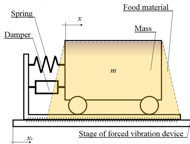
Figure 1. Approximated viscoelastic model of the food material.
