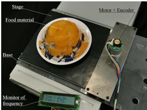
Figure 3. Prototyped forced vibration device.
