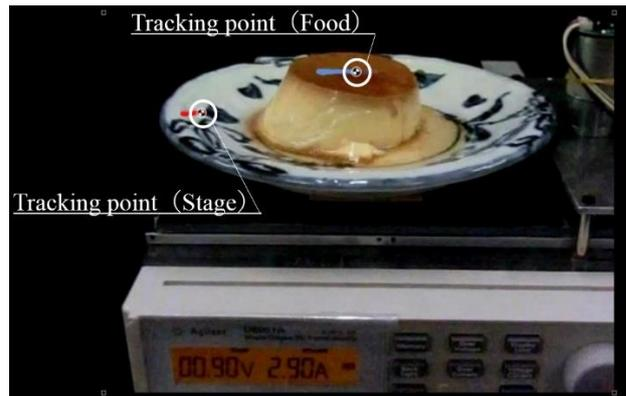
Figure 4. Measurement of phase difference and response magnification factor using image analysis.
