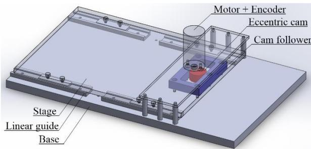
Figure 2. Concept of forced vibration device.
