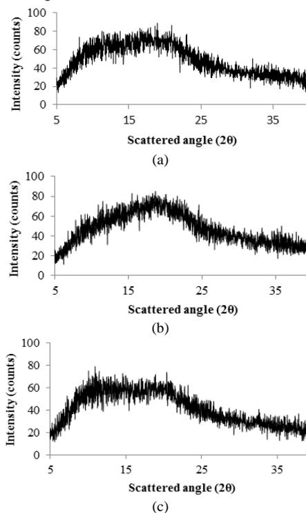
Figure 2. X-Ray diffraction scans of (a) non-process OSA starch, (b) spray-dried encapsulated powder and (c) freeze-dried encapsulated powder.
