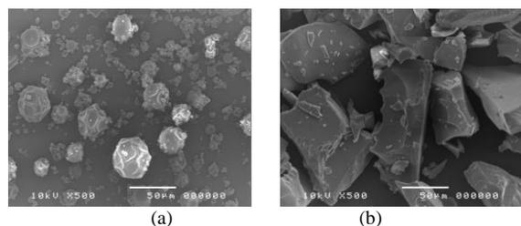
Figure 1. SEM photographs of microencapsulation of MAD flower extract using (a) spray drying and (b) freeze drying.
